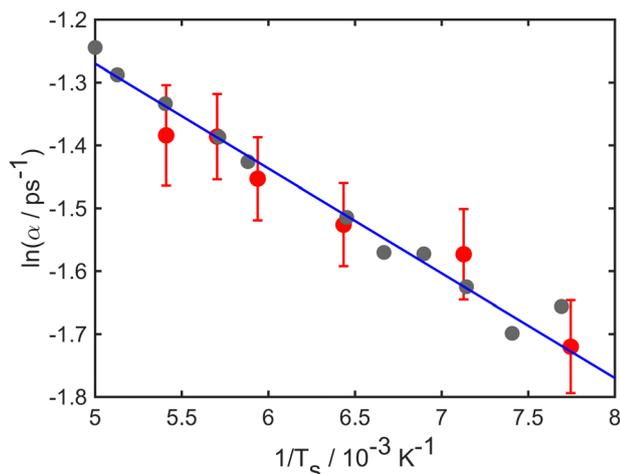
Fig. 2 Natural log of the decay rate  $\ln(\alpha)$ , as a function of the inverse temperature  $1/T$  for the Na–Cu(111) system with a momentum transfer  $\Delta K = 1.25 \text{ \AA}^{-1}$  for a corrugated surface with an energy barrier  $E_b = 55 \text{ meV}$  and a friction coefficient  $\gamma = 0.20 \text{ ps}^{-1}$ . Numerical results (grey points), experimental results (red points) and a linear regression line (solid blue line).
